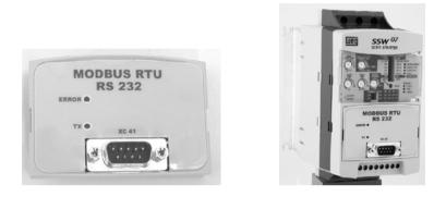
This interface enables the connection of the master to a Soft-Starter SSW-07/SSW-08 (point-to-point) at distances up to 10m. For the communication with the master you must use one wire for the transmission (TX), one wire for the reception (RX) and one wire for the reference (PE).
